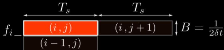
★ Perform a search in narrow frequency bands: sampling time  $\delta t = 1/2B$ , number of data points  $N_p = T_s/\delta t = 2T_s B$
